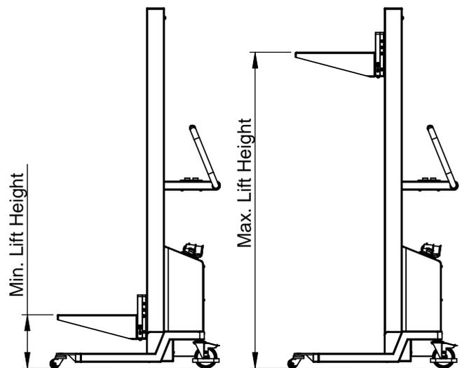
50C=50 dia swivel castors 100C=100 dia swivel castors 85P=85 dia pallet wheels 85R=85 dia Rocking Pallet Wheels
